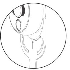
5) Using the included hex key, tighten the small hex screw until it flushes with the black ring (look at the picture on the right). Be careful not to cause its deformation.
