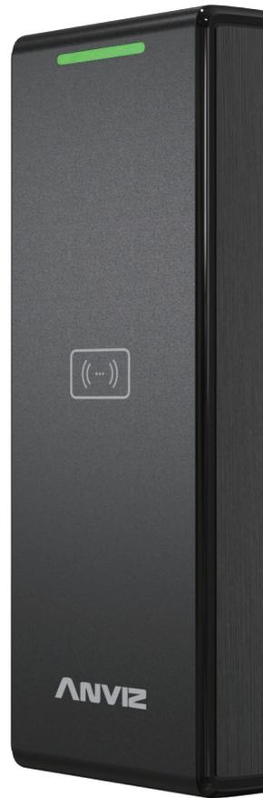
The C2SR device is a IP65 water- proof card reader, suitable for outdoor applications. It operates at 32-Bit High Speed CPU, supports 125KHz EM card or 13.56MHz mifare. The C2SR has Wiegand 26/34, with operating temperature of -20°C~65°C and operating humidity of 20%-80%.
