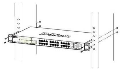
Figure 5 - Mount the Switch in the rack or chassis
