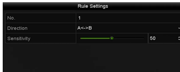
Figure 10-6 Set Line Crossing Detection Rules
