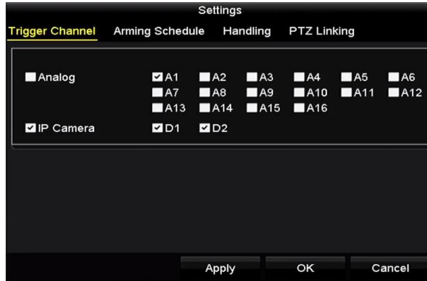
Figure 9-15 Set Trigger Cameras of POS
