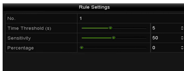
Figure 10-8 Set Intrusion Crossing Detection Rules
