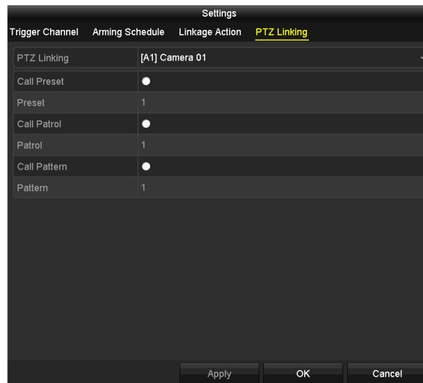
Figure 8-7 Set PTZ Linking of Alarm Input
