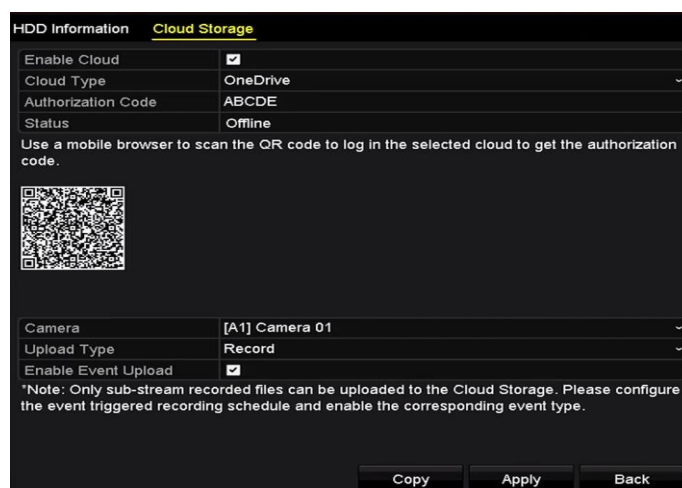
Figure 14-20 Upload to Cloud Storage Interface
