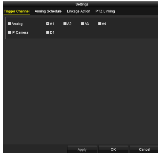
Figure 5-23 Set Triggered Camera of VCA Alarm
