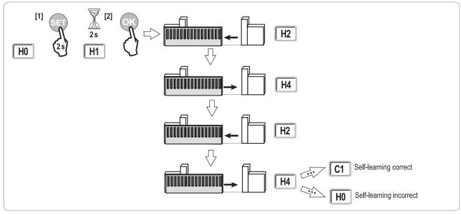
If self-learning starts when the gate is closed, stop the self-learning in progress (press a control button: motor electronics, memorised remote control, wired control point, etc.), move the slide as shown opposite, then restart self-learning.
