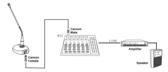
B: Connect the microphone to audio console
